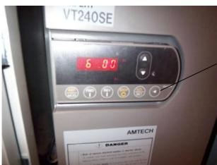
Push the Arrow Button to move the flashing digit to the digit to the right of the six.
