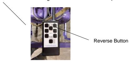
The machine must be moving to turn. Start the machine moving then press the Left Steering Button on the remote control. The machine will turn to the left. Let up on the button, the turning will stop and the machine will continue in a straight movement.
