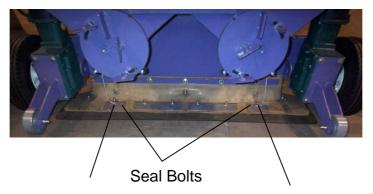
The overlap for each pass depends on the application, thickness of paint, etc.. In general you want to line up the first bolt on the seal with the cut line of the previous pass.
