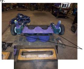
Unbolt the gear box from the support bracket.
