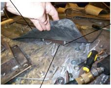
Step 1- Lay the Retainers out on a flat surface with the threaded studs facing upward. Place the black Main Seal down over the studs. Make sure that the tapered edge on the main seal is down facing the floor.
