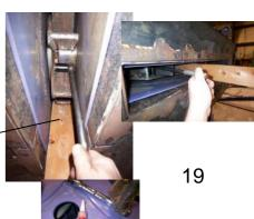
Remove the two end liners by removing the nut on the end wall of the Blast Cabinet. Tap the end of the threaded stud to loosen the liner.
