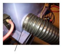
Connect the other end of the exhaust hose to the dust collector. Leave the clamp loose, for now; the hose will have to be adjusted to remove twists and loops after the fan is started.
