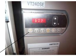
If the speed is set at 60 cycle, push the Mode Button and the display will flash showing the A00-0 cycle parameter set point.
