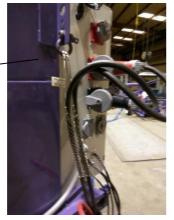
Plug in the blast machine wiring harness. Connect the cable support slings to a shackle on the dust collector. This keeps slack between the sling and the plugs so wires are not pulled loose when moving the dust collector.
