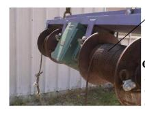
Make sure that the cable wraps on the hoist drums are straight and smooth across the drum.
