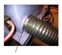
Connect 75' of standard exhaust hose to the dust collector.
