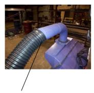
**Caution-** Connect 20' of High Temp Exhaust Hose to the machine exhaust elbow and secure with a hose clamp.
