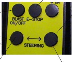
**Steer Right** Bump or tap the button too make slight steering corrections. Hold down longer for turning.
