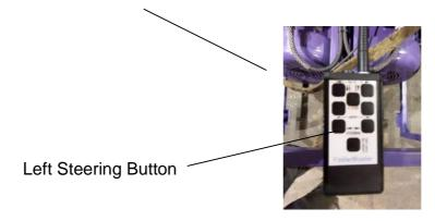
Press the Right Steering Button on the remote control. The machine will turn to the right. Let up on the button, the turning will stop and the machine will continue in a straight movement.
