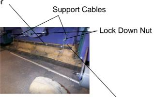
Step 8- Install the four Support Cables from the corner retainer studs to the lock down coupling nuts on the Blast Cabinet, as shown. The cables should be slack enough to allow the seal to float, but tight enough to support the seal assembly when the machine is lifted off the ground.
