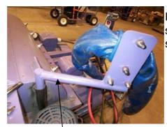
Remove the cable harness support by lifting it out of the support tube.
