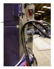
Plug in the blast machine wiring harness. Connect the cable support sling to a shackle on the dust collector. This keeps slack between the sling and the plugs so wires are not pulled loose when moving the dust collector.
