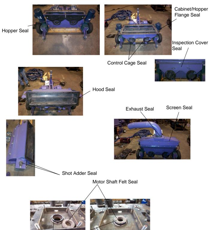
Glue the felt seal in place with silicone
