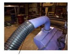
Connect the exhaust hose to the exhaust elbow and secure with a hose clamp.
