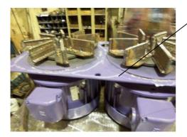
Place a bead of silicone all around the wheel mounting plate as shown.
