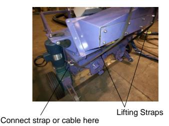
Set the machine up from the horizontal position to the vertical position. Make sure that the Support Stand Assy is in place and bolted down securely. Attach lifting straps or the hoist cables to the side lifting lug on each side of the machine. Run the straps under the hopper and in front of the exhaust hood as shown. **Caution-** keep personnel away from the machine and lift slowly. The machine will flip up to the vertical position.
