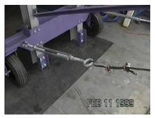
Run the cable from the turnbuckle through the rear eye and around the tanks center stand pipe. Run the cable back through the other rear eye and connect it to the opposite turnbuckle, using at least two 3/8" cable clamps. Pull the cable tight as possible before clamping. Next, pull the two cables together and place a single clamp about two foot from the stand pipe. This will keep the fixture running square to the tank.
