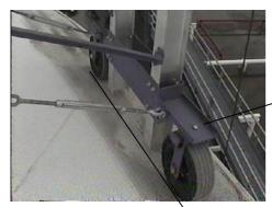
Make sure that the wheels are straight in line with each other rather than turned to match the radius of the tank.
