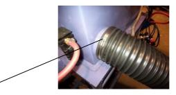
With the fan running, rotate all twists and loops out of the exhaust hose. The hose must be straight to minimize damage and pressure drop. If the suction of the dust collector is too great to rotate the hose, turn Off the fan and rotate the hose as the fan slows down.
