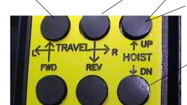
Press and hold for **Right Travel** of the fixture when in vertical mode- release button to stop.
