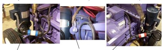
To pick up the machine, place a lifting strap on each side of the machine using a 5/8" shackle in the lifting lugs shown above. The machine is balanced at this point so it will be level.
