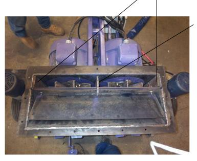
The Center Liner must be removed by driving it up from the bottom side of the blast cabinet with a hammer. Fill any wear areas with hard face welding rod and reinstall by driving it down from the top side of the Blast Cabinet. Drive it down into the notched cutout in the cabinet and the pocket in the Hopper. Be sure to center the bottom of the liner equal distant from the two Blast Wheels. Tap the liner bottom end to the right or left to center it between the two sets of blades.
