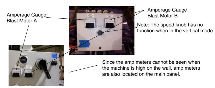
Adjust the shot flow to bring the amperage up or down to approximately 35 amps. See pages 31 & 32 for adjustment procedure.
