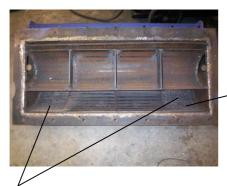
Remove the Top Curved Liners and fill any wear areas with hard face weld. If the wear is too great, replace the liners.
