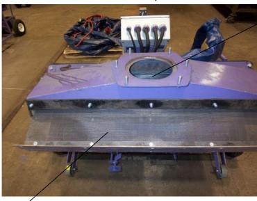
To inspect the screen, remove the exhaust elbow and view the condition of the screen through the round opening.
