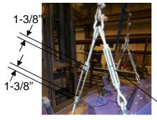
Connect the short 3/4"x9" turnbuckle on the lifting lug located on the Hood Assy. Use a 5/8" shackle.
