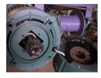
5. Slip the brake assembly off of the motor shaft being careful not to pull on the brake electrical wires. Support the brake to prevent stress on the wires while cleaning the brake.
